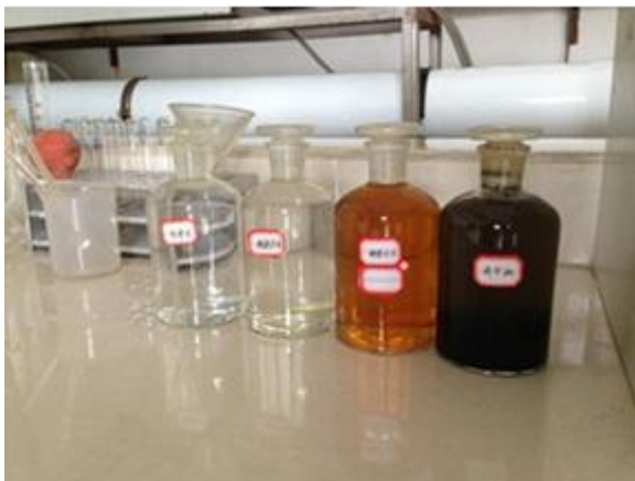
From left to right: leachate-anaerobic-aerobic-nanofiltered- tap water
