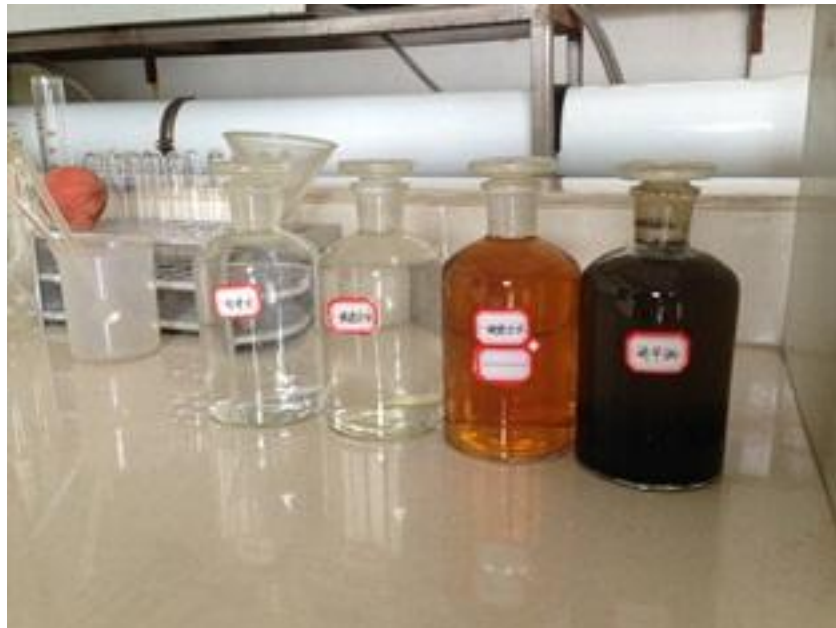
Figure 5-9 From Leachate to Effluent - Leachate Treatment in Xishan Incinerator
