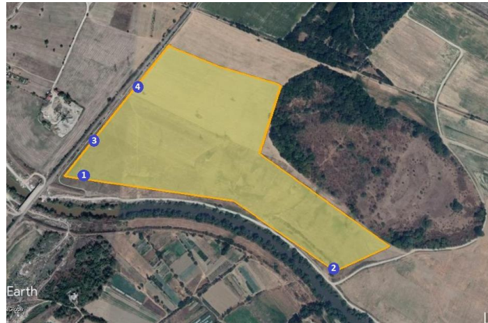
Figure 10: Noise Level Measuring Points around the WWTP Site
