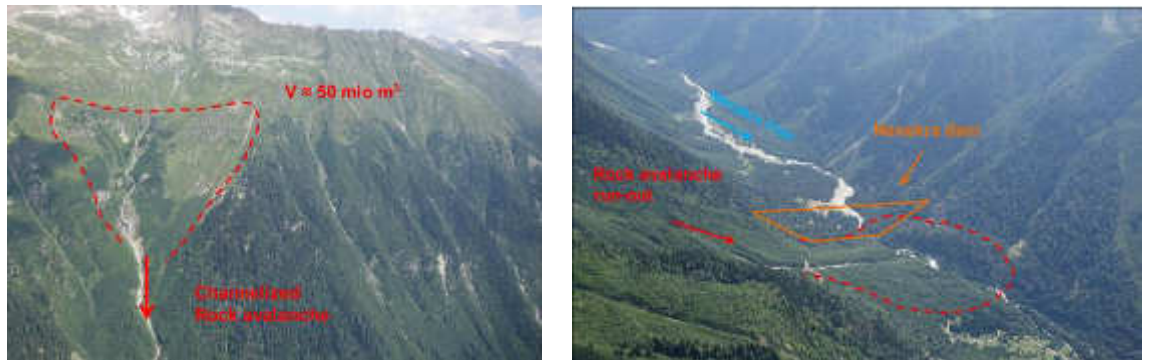
Visual evidence of an historical landslide deposit at the dam emplacement. Left: View from the left bank towards the detachment zone of the landslide event. The volume of the material is probably significantly less than 50 million cubic metres. Right: Maximum extension of the landslide and run-up area on the opposite slope.
