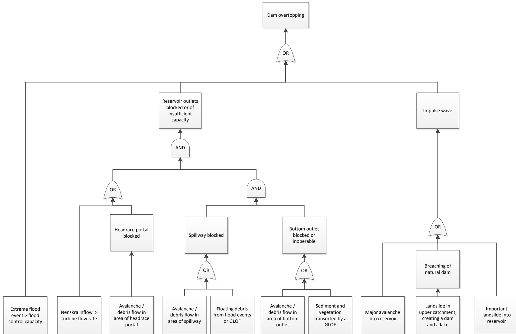
Figure 18 – Fault tree for dam overtopping during operation
