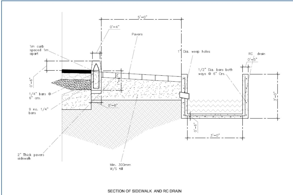
**Figure 2-5: Cross Sectional view of the Sidewalks and Reinforced Concrete Drains<sup>3</sup>**
