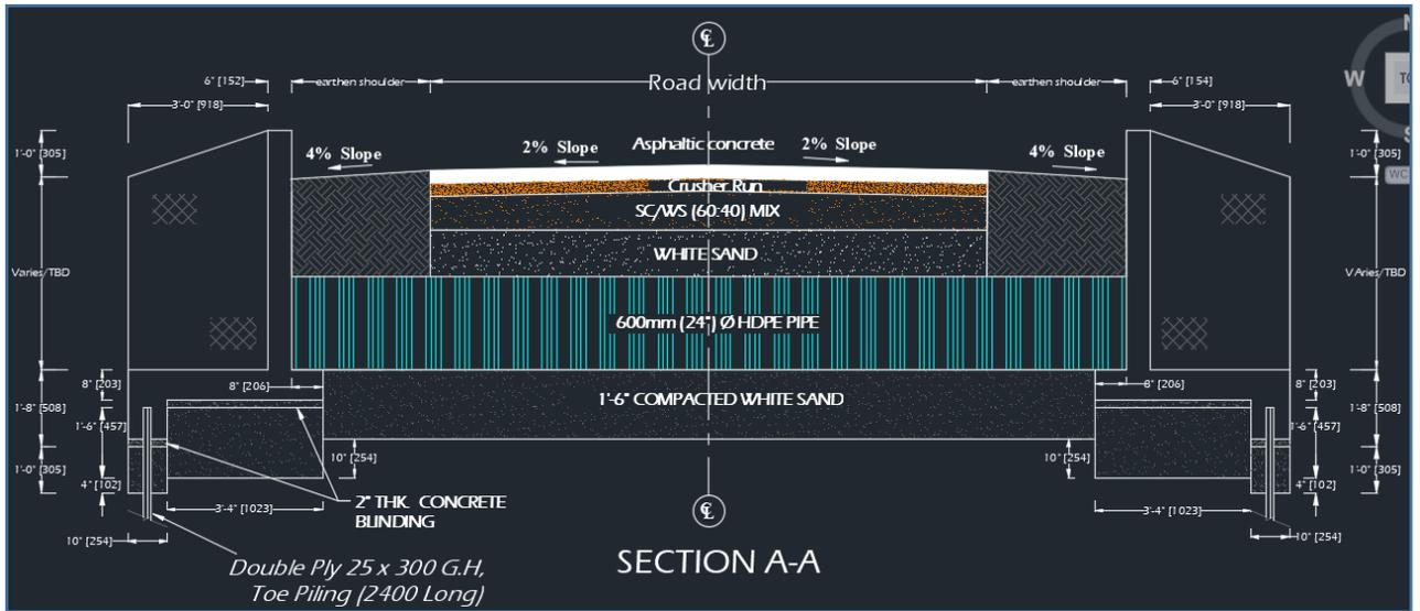
Figure 2-7: Cross Section of Culvert<sup>4</sup>
