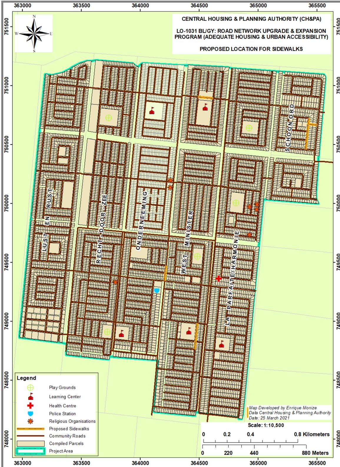
**Figure 2-4: Map showing the Locations of Sidewalks that are to be constructed**
