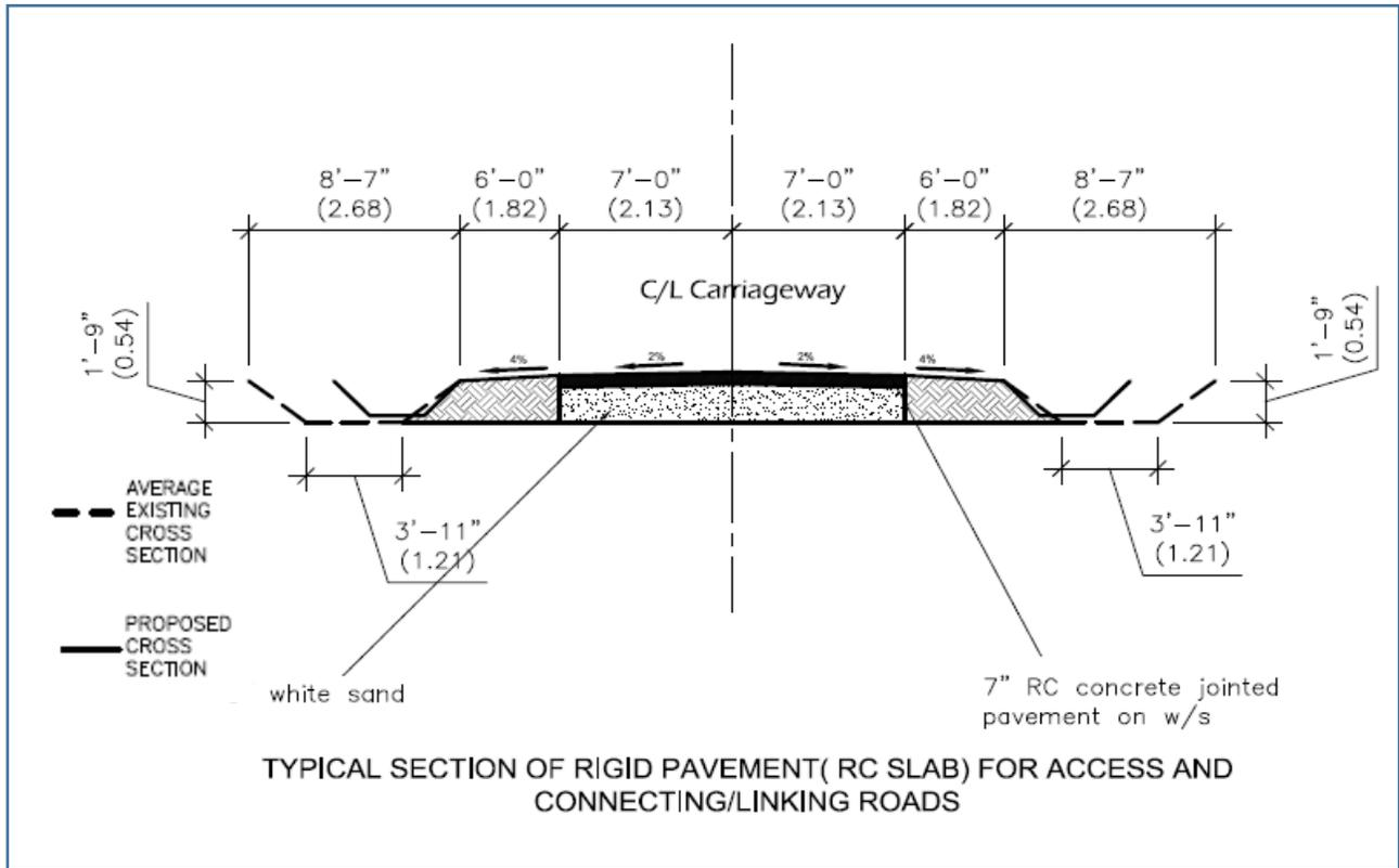
**Figure 2-2: Typical Section of Rigid Pavement for Access and Connecting/Linking Roads<sup>2</sup>**
