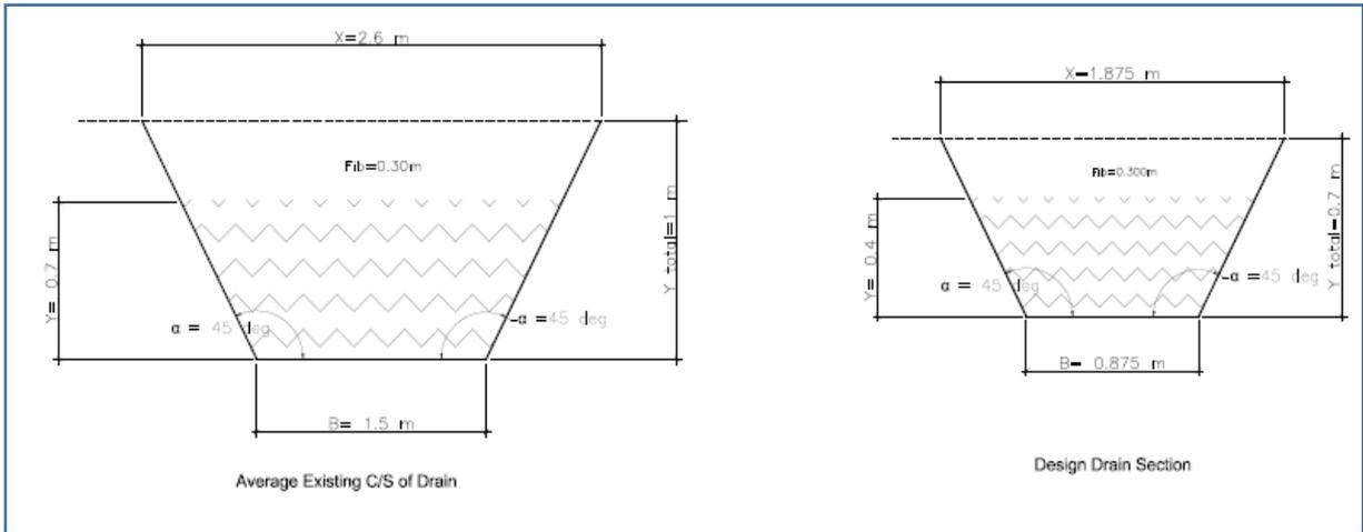
**Figure 2-8: Cross Section of Earthen Drains/Canals<sup>5</sup>**
