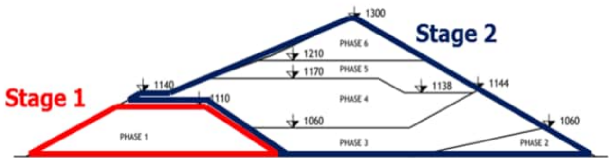
Figure 3-3 - Overview of Construction Stages and Phases
