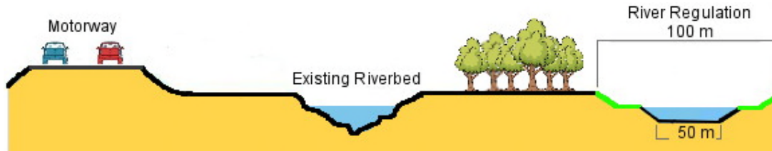
Figure 3-7. Typical Cross-Section of the Regulated Channel
