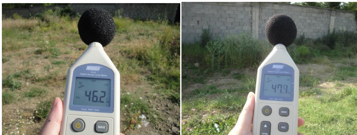
Figure 17 and 18: Noise level measurement at “Narimanov” and “Marneuli” reservoirs
