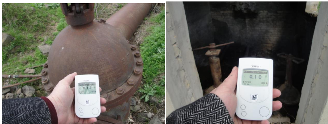
Figure 15 and 16: Measuring the radiation background in the Nerimanov reservoir project area
