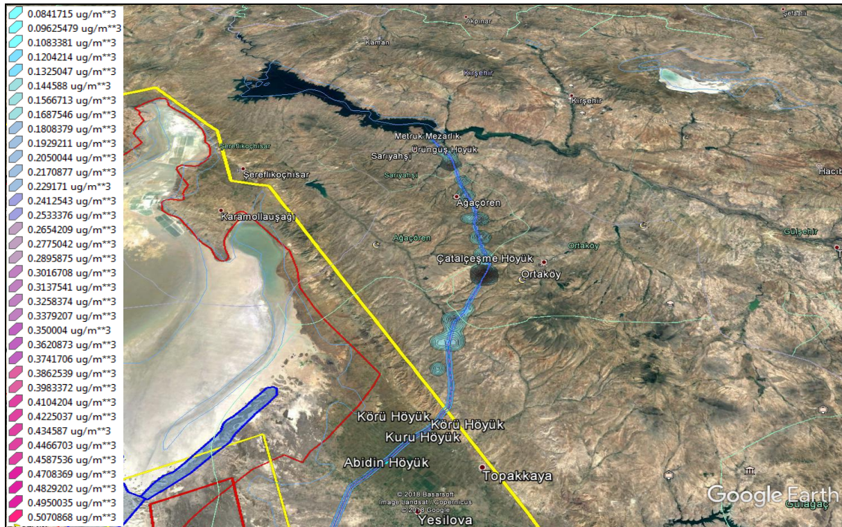
Figure 5.6.2.8 Profiles showing the annual distribution of PM10 values resulting from the model 2 (0,55 \mu\text{g} / \text{m}^3 )
