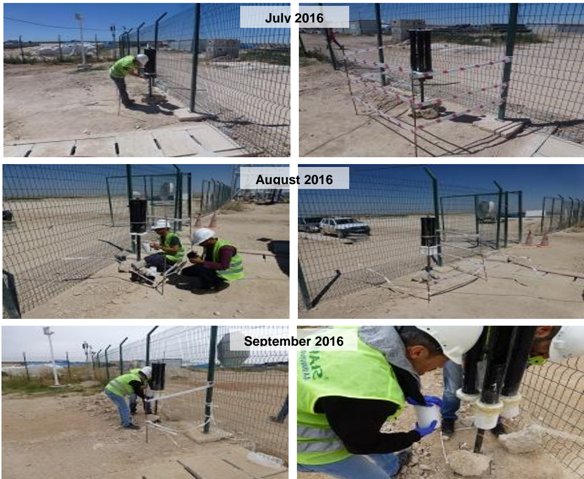
Picture 4.3.2.1. Photos of Air Quality Measurements (Dust Deposition, PM 10 ) at the Project Sites
