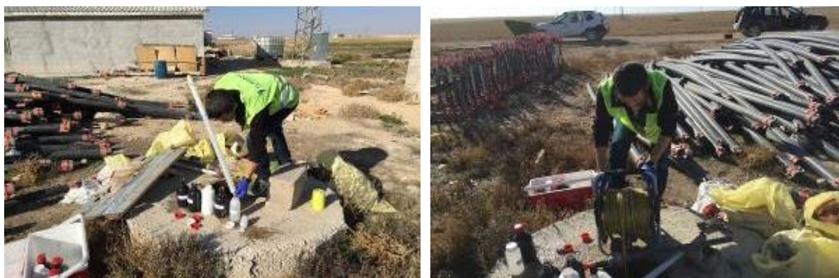
Picture 4.9.3.1. Groundwater Sampling and Water Level Measurement at GW-1 Sampling Point for the EIA Baseline Studies
