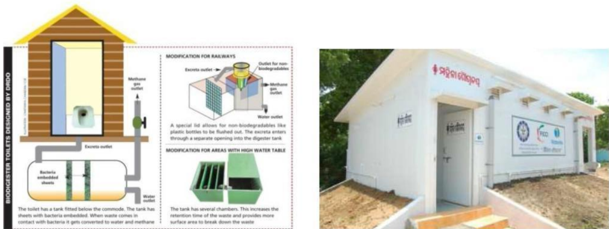
Figure 8.2: Typical Cross Section of Bio Digester
