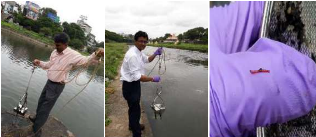
Insertion of Vanveen grab for sediment collection
