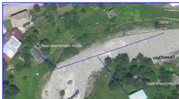
Fig. 12: Route of outfall collector (1) and nearest users downstream
