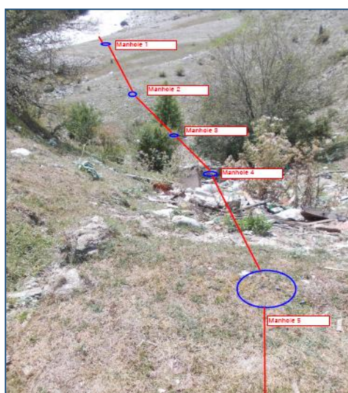
Fig. 18: Route of outfall collector (4) after the collective septic tank
