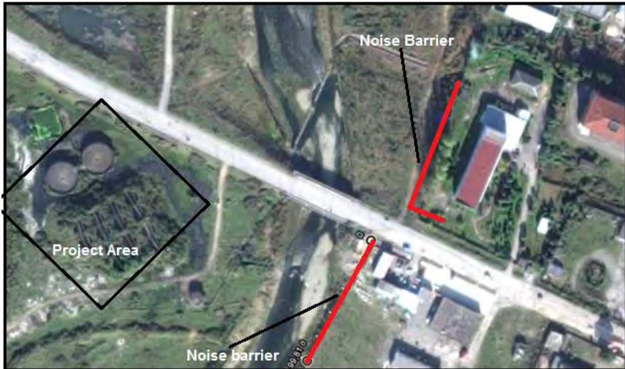
Figure 12 - Noise Attenuating Barrier at the sensitive receptors
