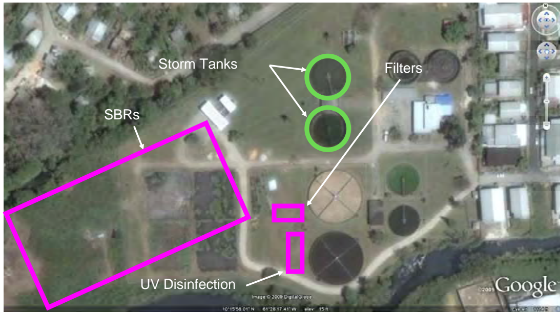
Figure 4-9 Conceptual Site Layout of Option L4
