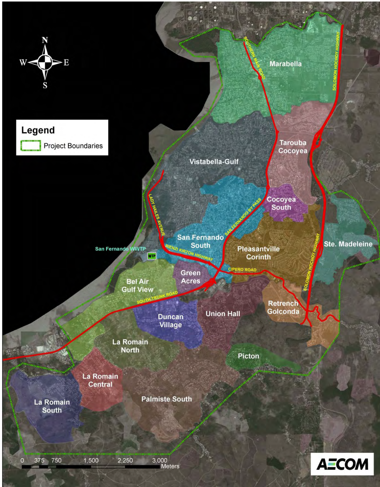
Figure 6 Subcatchments of the San Fernando Wastewater Project
