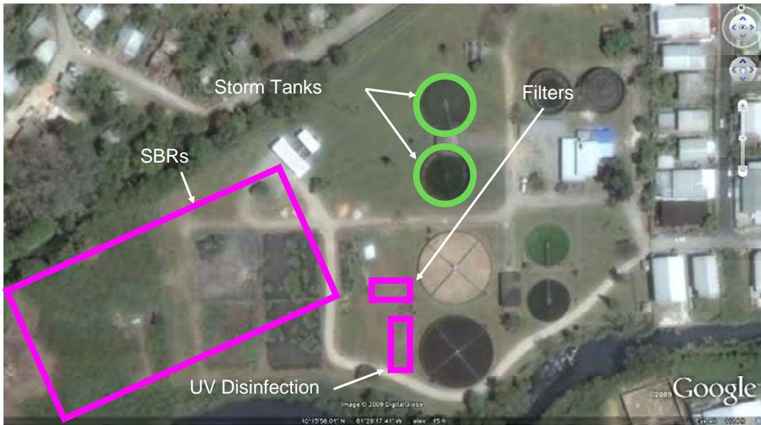
Figure 4-9 Conceptual Site Layout of Option L4
