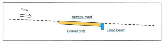
Figure 8: Typical Detail - Gravel Drift
