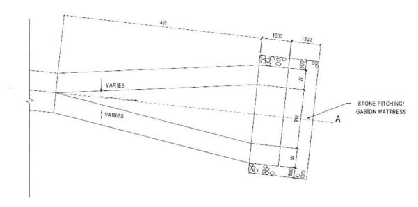
Figure 12: Typical Detail - Outlet with Erosion Protection
