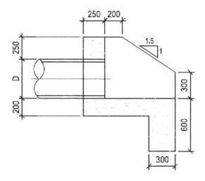
Figure 11: Section through Typical Inlet/Outlet Structure
