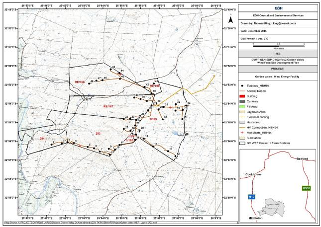
Figure 3.2: Site Layout of the Golden Valley Wind Energy Facility
