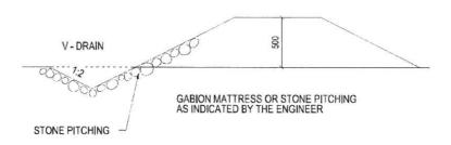
Figure 9: Typical Detail - Berm
