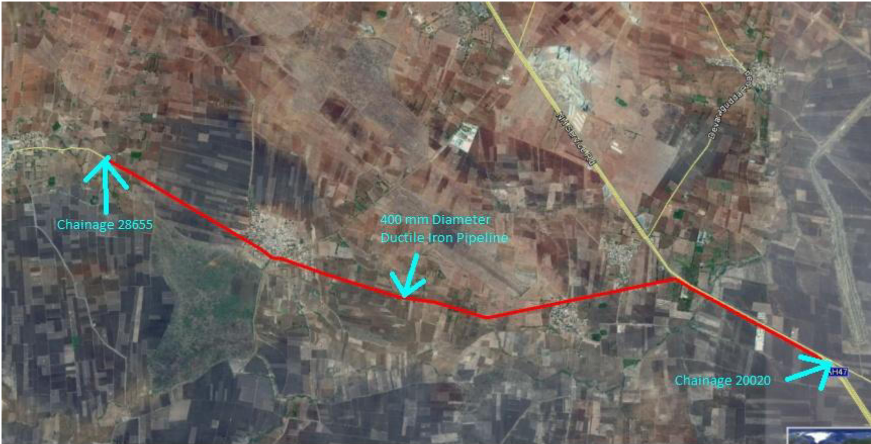
Figure 5: Proposed 8.7 km Raw Water Transmission Alignment
