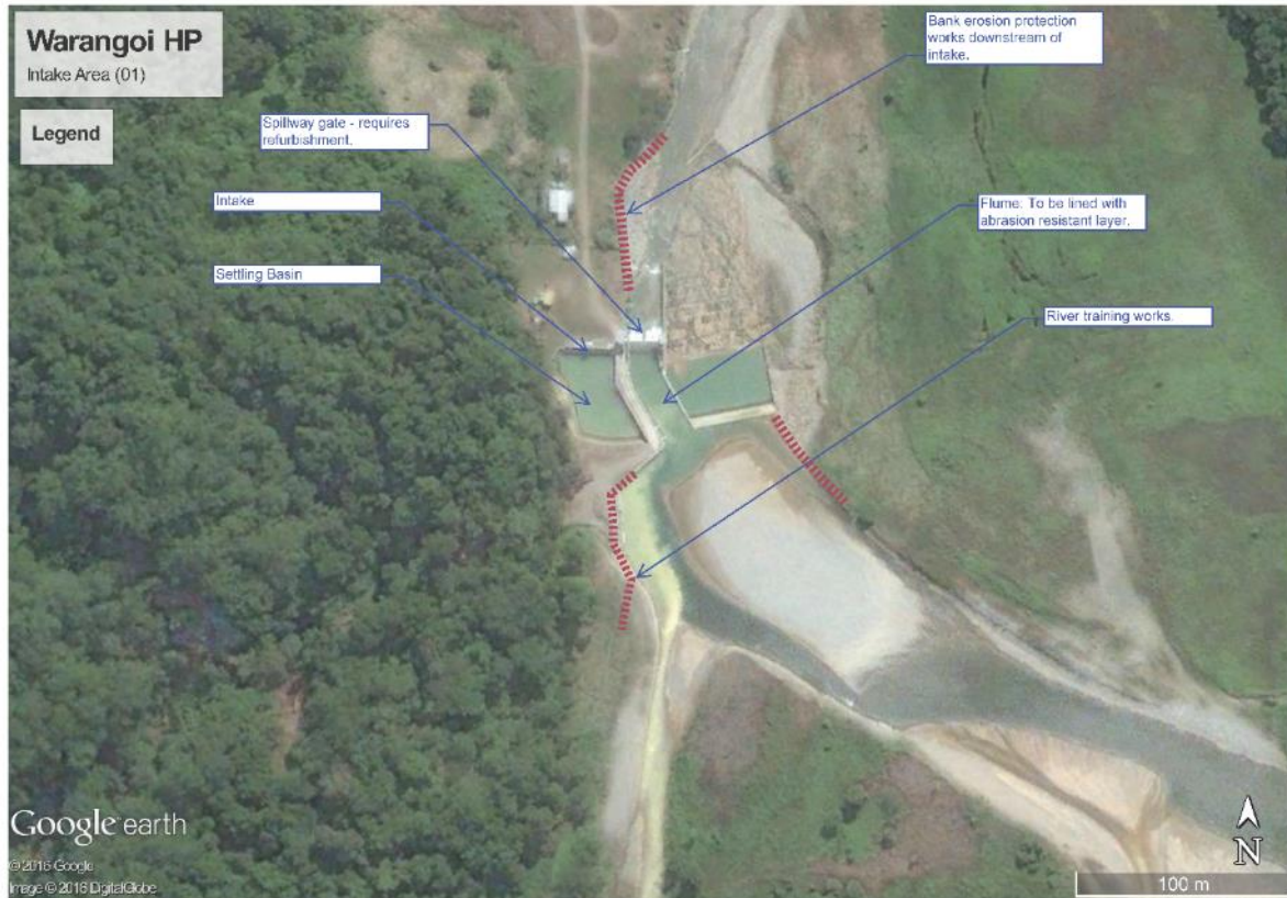
Figure 5 Warangoi HP proposed intake and river protection works
