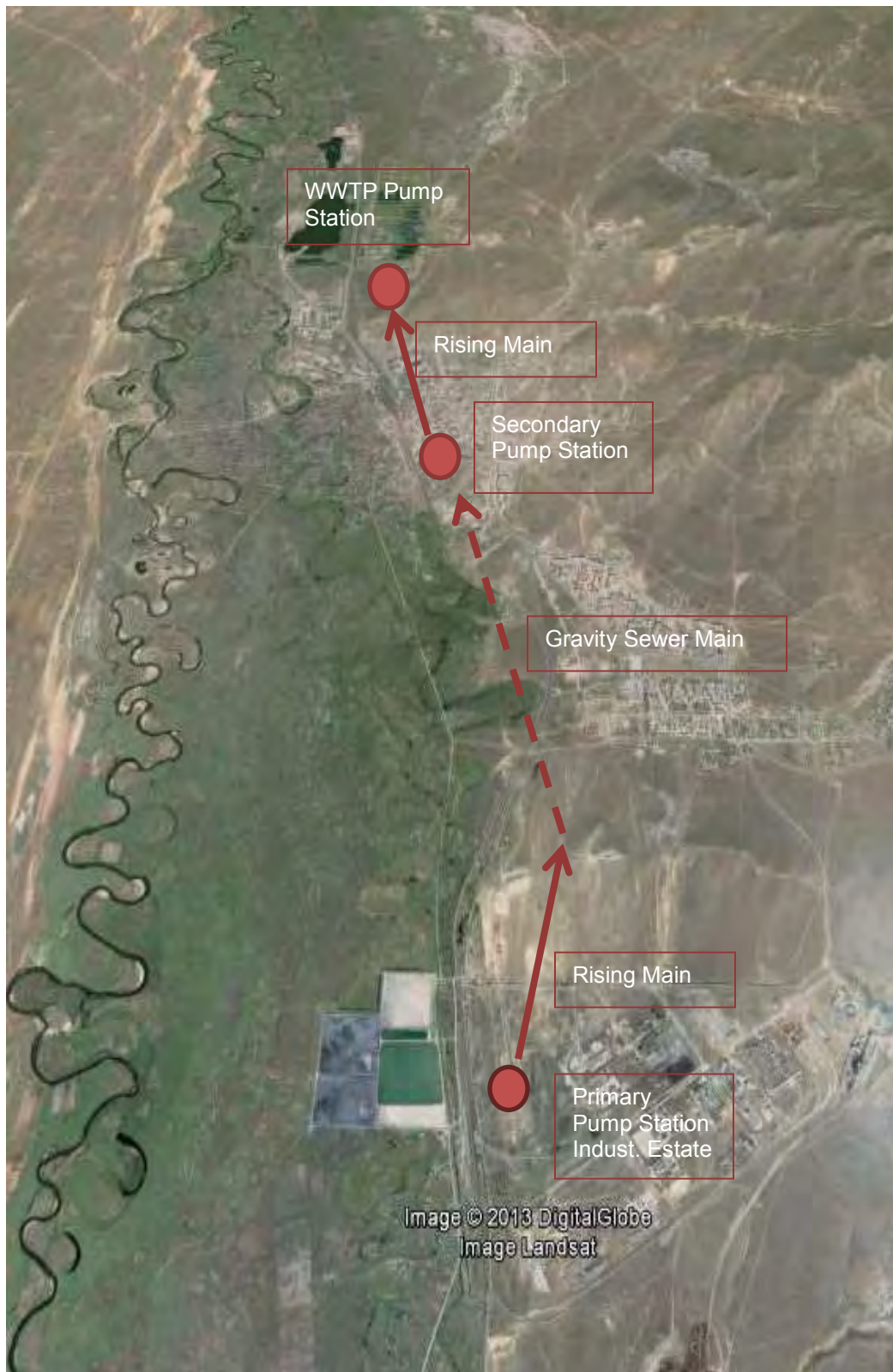
Figure A1.3: Arrangement of Sewage Pumping Stations
