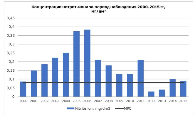
Figure 5.8: Annual average concentrations of nitrite ion in River Svisloch, mg/dm<sup>3</sup> (Korolischevichi)
