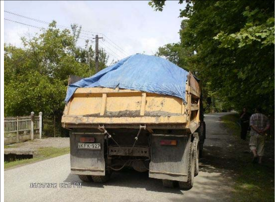
Backfilling material protected by tarpaulin.
