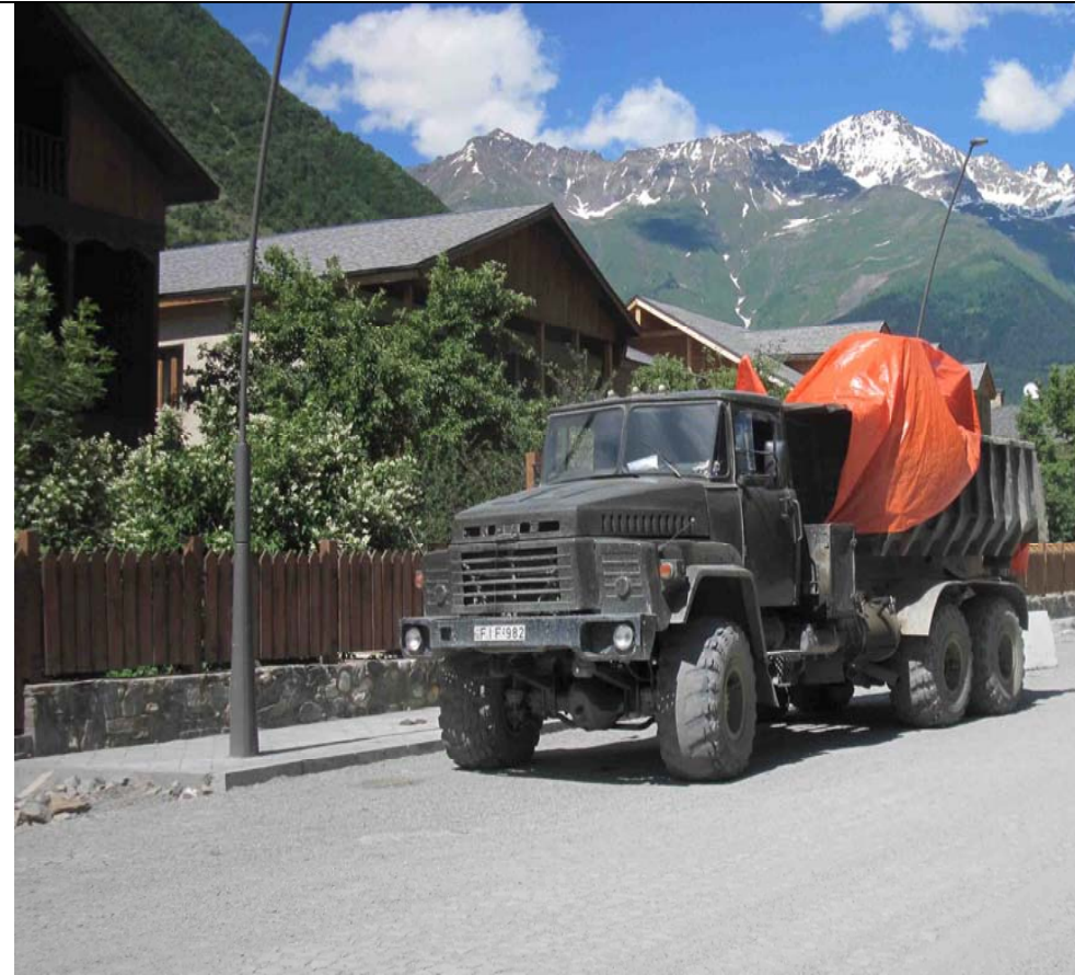
Photo No. 14 Tarpaulins are used to cover loose materials that are transported to and from the site by track.
