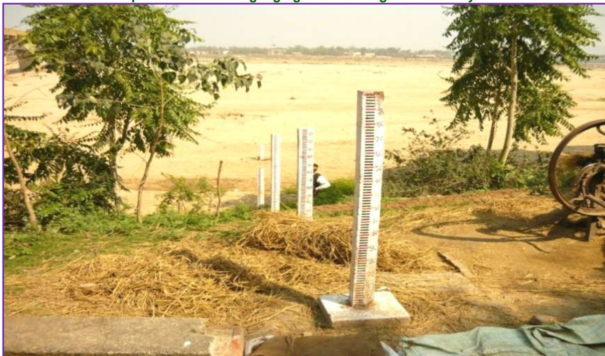
Photoplate-10.1. Stream gauging station being monitored by CWC
