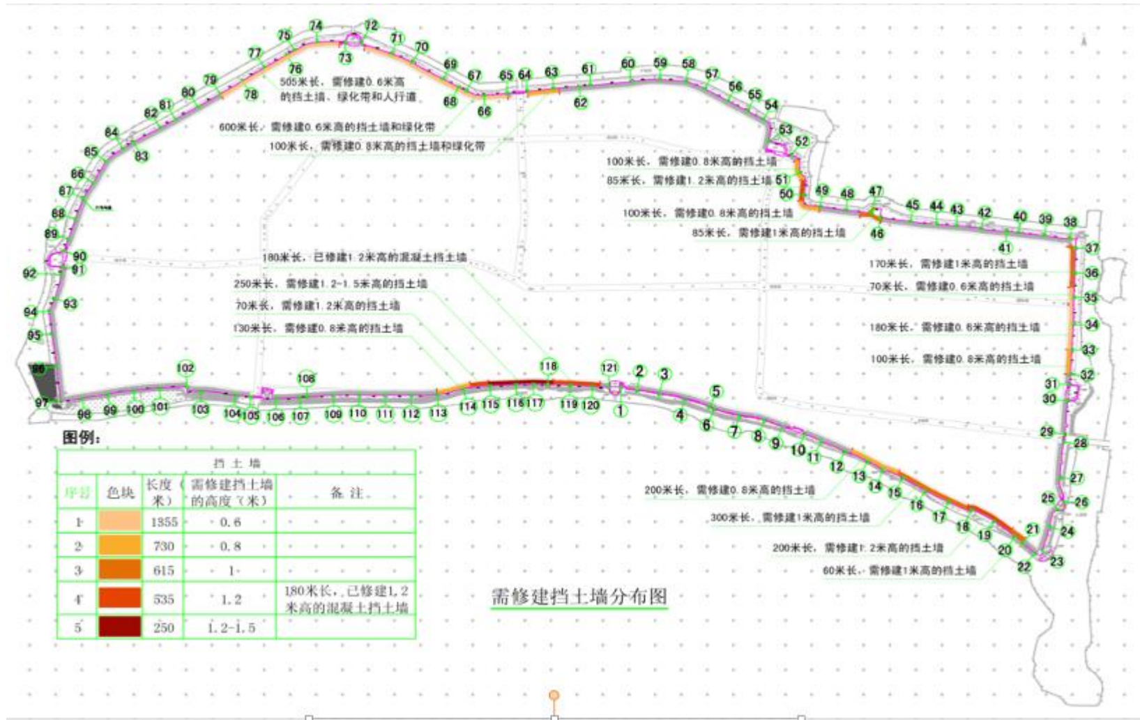
Figure 3.3-2 Distribution of retaining wall
