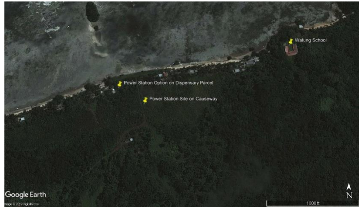
Figure 14. Google Earth image showing proposed location of the power station and battery house within the existing road and utility easement underlying the causeway (center) in Walung. The alternate site on the dispensary property is also shown (left) along with the location of the school (right).
