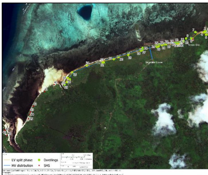
Figure 12. Google Earth image of Walung village in northwest Kosrae with digital overlays identifying residences to be connected to the mini-grid (yellow dots) and residences to receive SHS (red dots). The proposed site of the small power station is in the middle of the blue line, which demarcates the unimproved Walung causeway. Two other residences now to be added to the mini-grid, but not shown here, lie at the inland terminus of the causeway (blue line).
