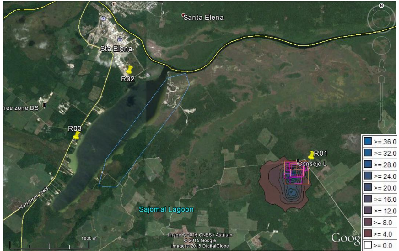
Figure 54 – Spatial distribution of CO diffusion ( \mu\text{g}/\text{cm} )
