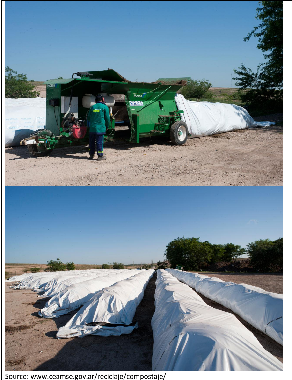
Figure 29 – Plastic membrane biotunnel composting
