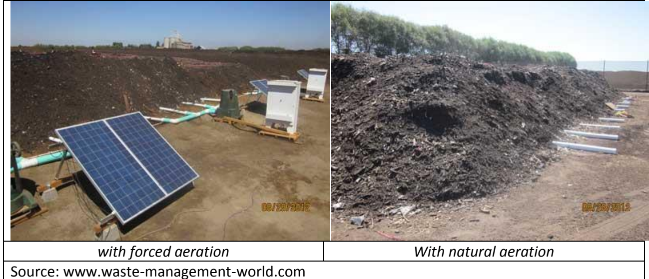
Figure 30 – Static windrow composting
