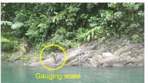
**3E.** Gauging station – limnimetric scale
