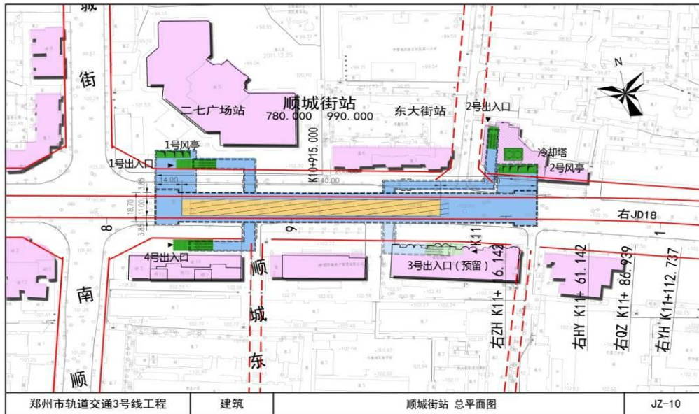
Fig. 1-3: The demolition of two residential buildings is avoided in the optimized design scheme, which saved a cost of RMB 60million Yuan for resettlement
