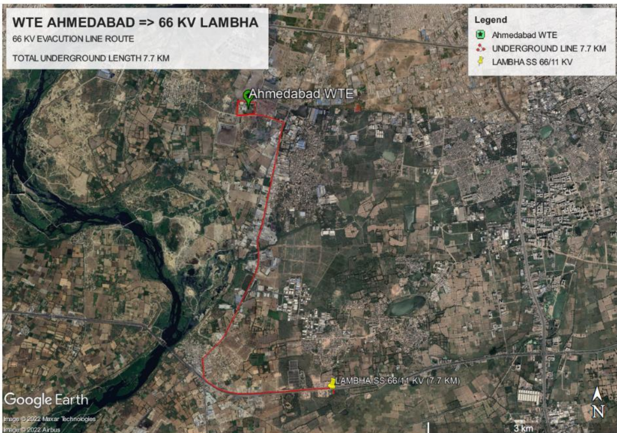
Figure 2-7 Transmission Line Route
