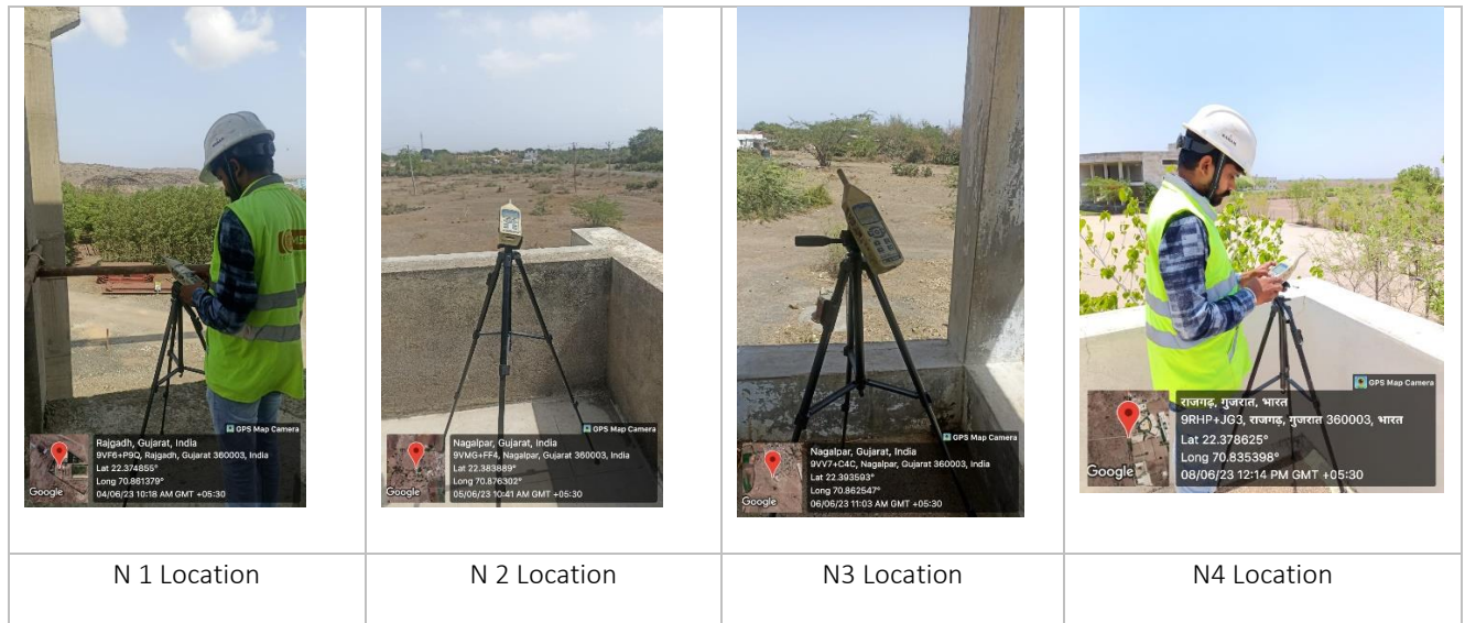
Figure 5-20 Noise Level monitoring conducted in Study Area
