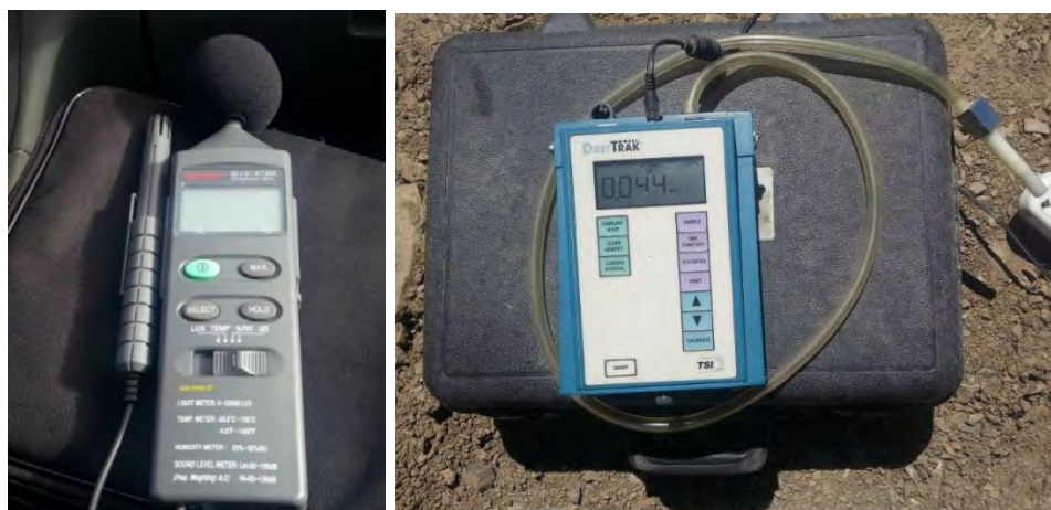
Figure 25: Noise dust measurement devices used for monitoring
