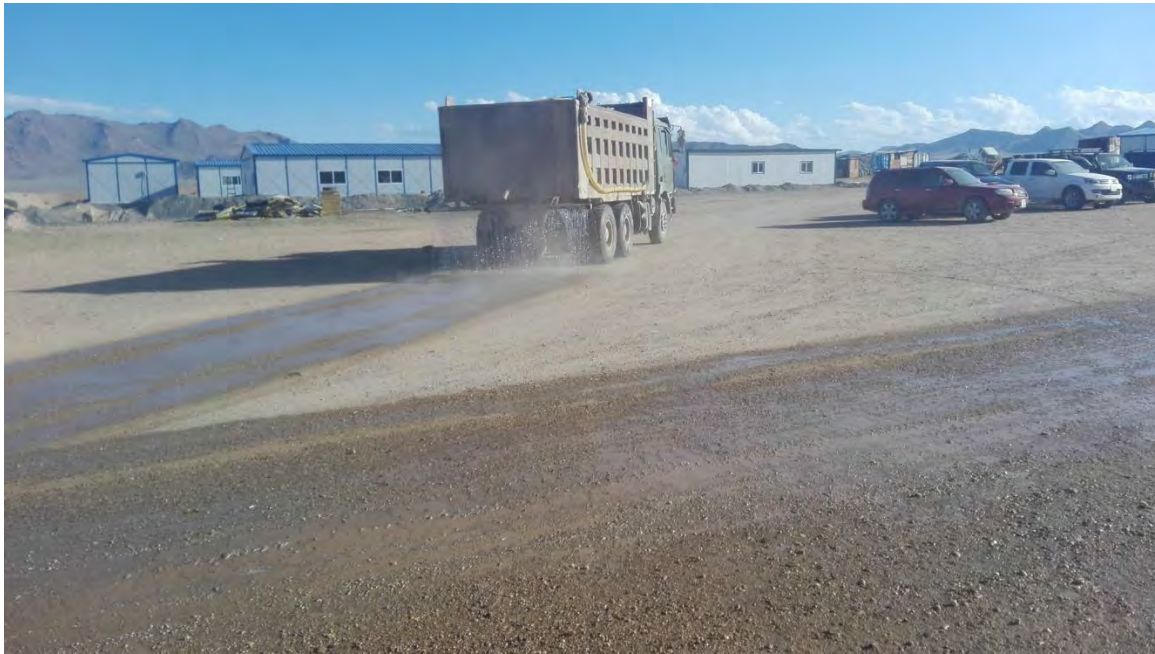
Figure 7. Water spray truck, CW1-2.
