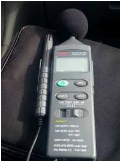
Figure 11: Noise measurement device used for monitoring
