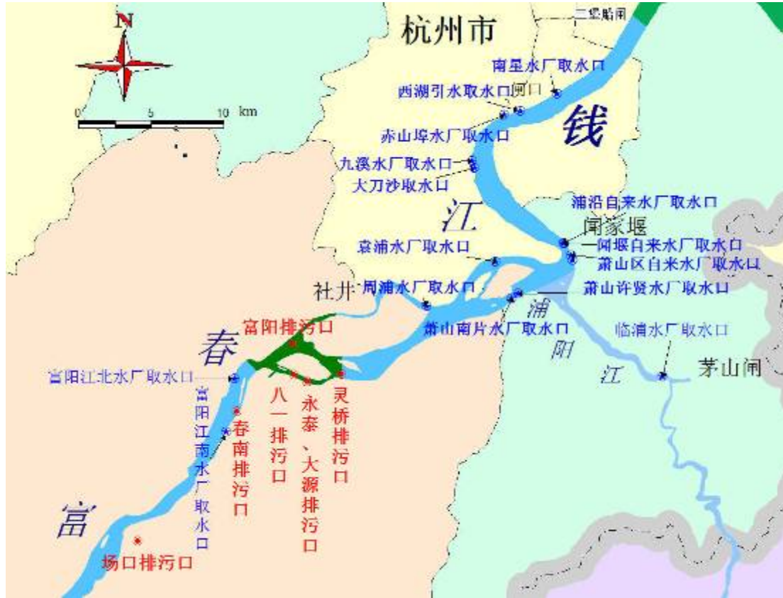
Figure 1.6-1 Layout Drawing of Discharge Outlet and Intake along the Fuchun River, the Water Body Absorbing Pollutants from the Stage IV of Fuyang Sewage Disposal Project
