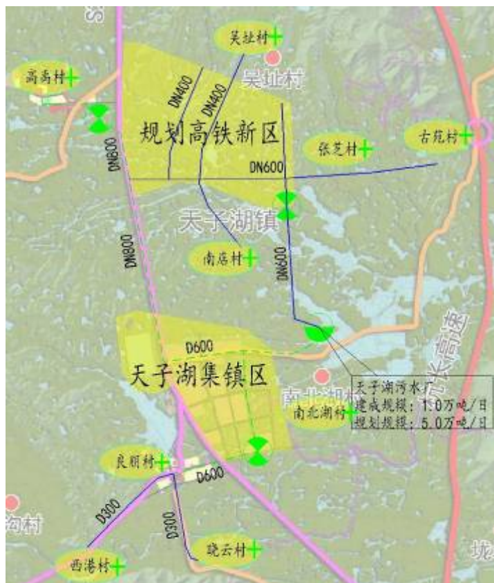
Figure 3.1-1 Layout of Drainage Network of Anji Tianzihu District
