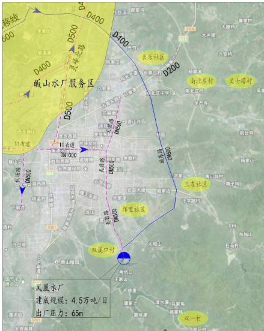
Figure 3.1-11 Construction Schematic Drawing of Water Supply System of Anji urban area
