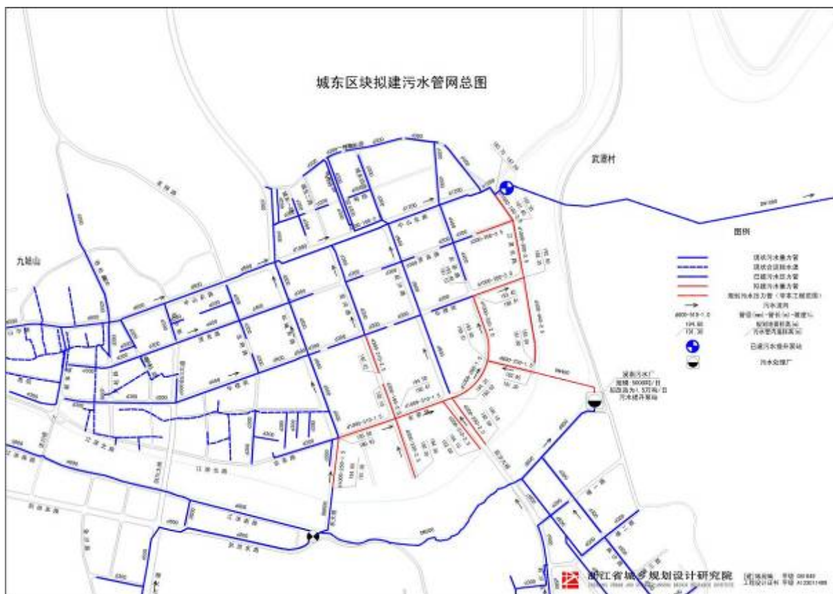
Figure 3.3-3 Layout Drawing of Sewage Pipe Network of Longquan Urban Area
