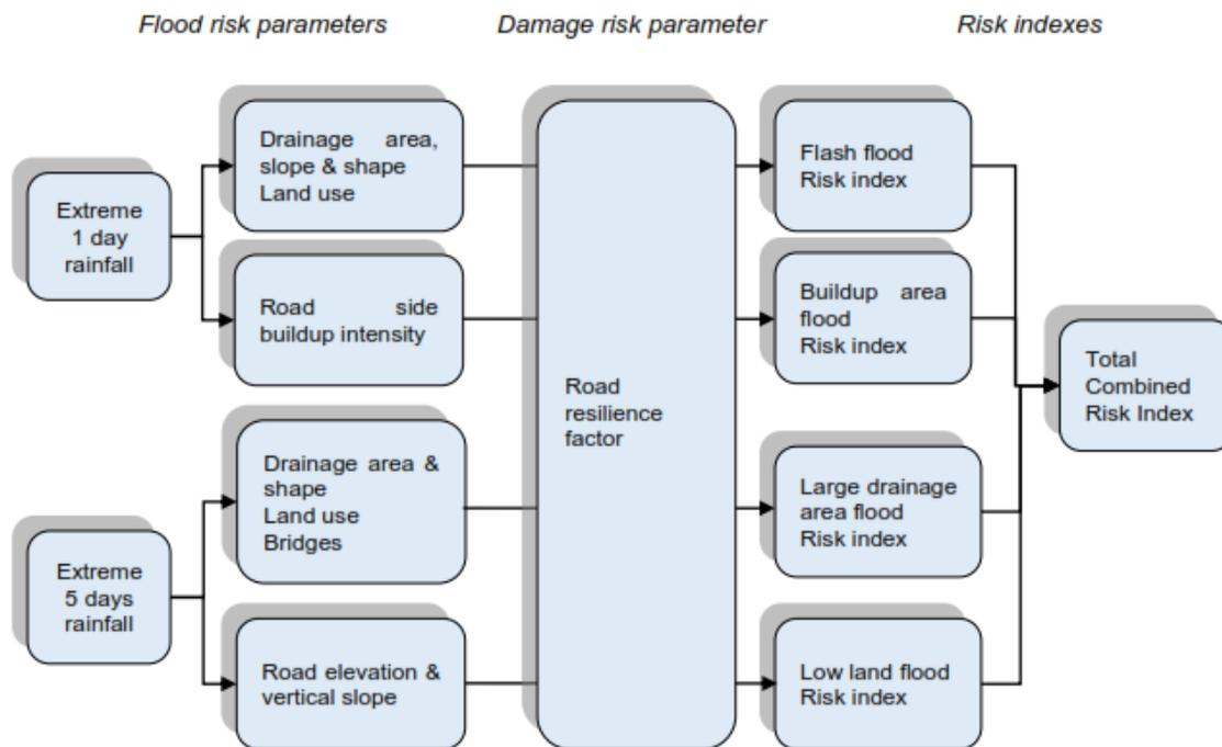
Figure V-1 Flow Chart for Derivation of Flood Index
