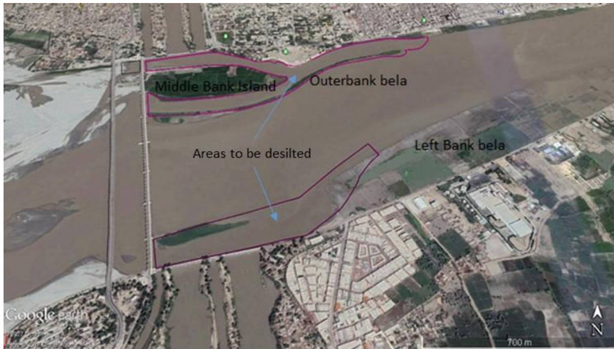
Figure 3.2: Locations of the areas to be desilted in the barrage
