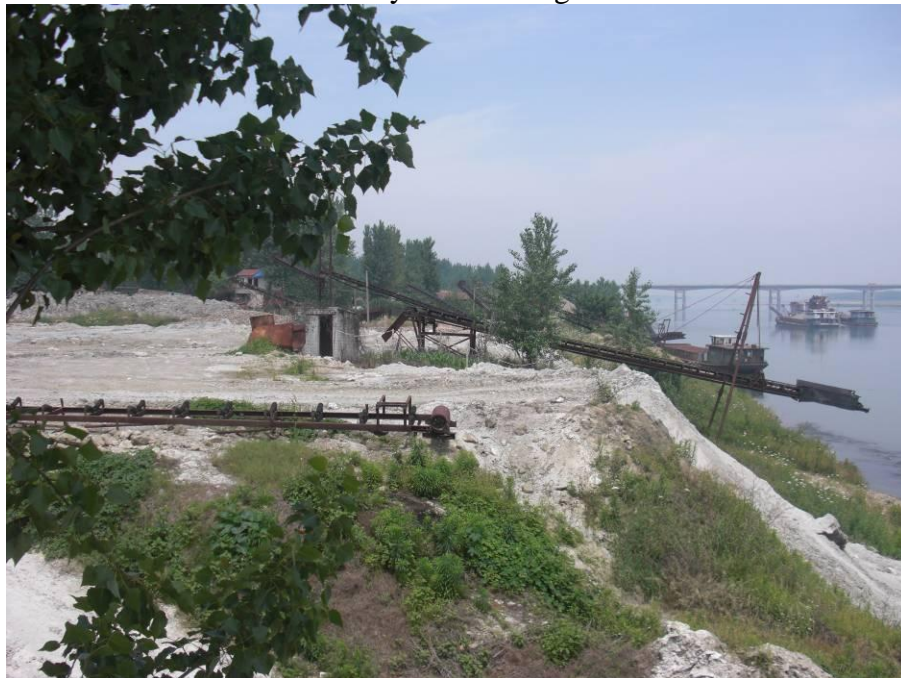
Figure 2-15 Sandstone-transporting equipment of Xiangyang Yonghongji Concrete Co., Ltd. needs to be heightened after water storage
