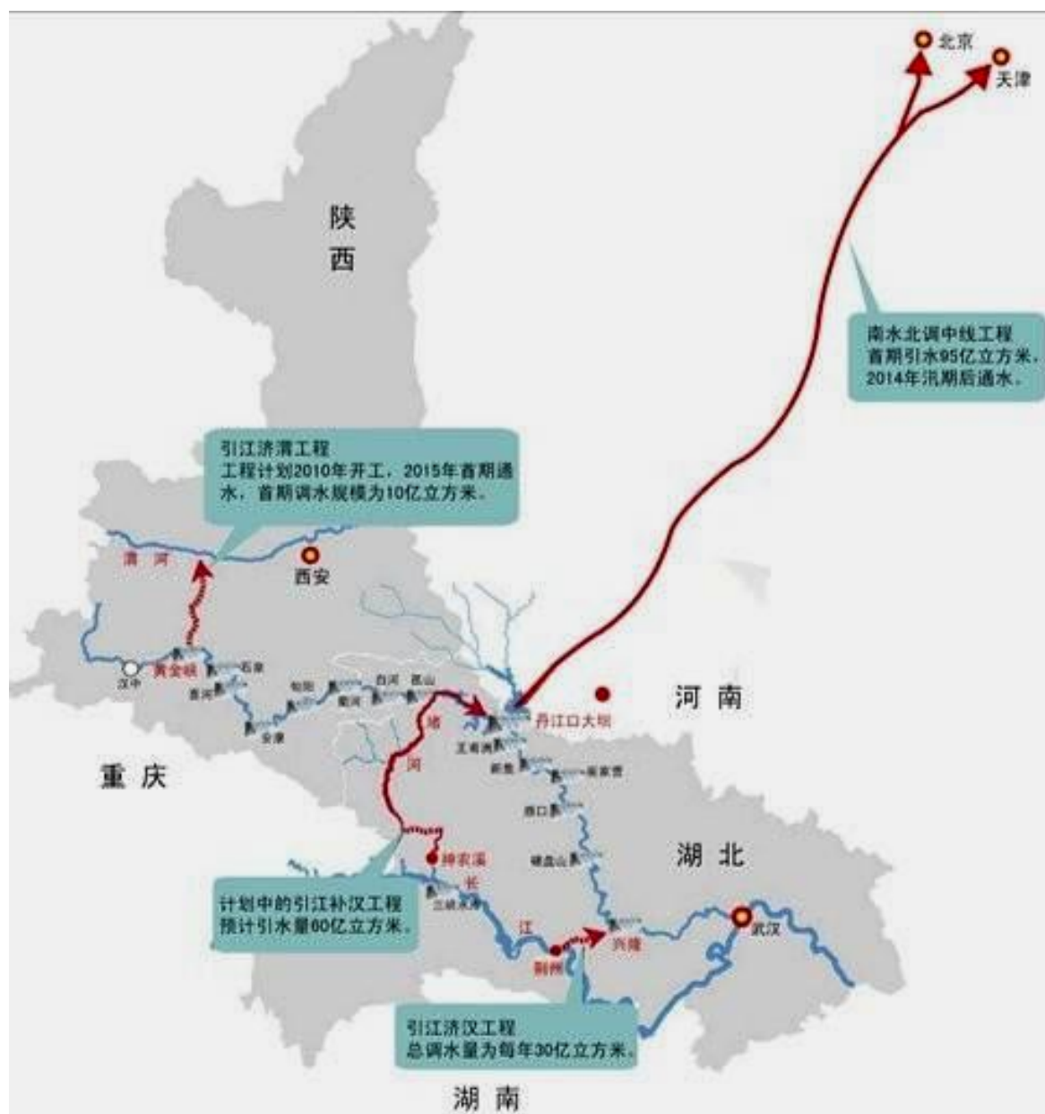
Figure 2.1.2-3 Sketch map for the 1st stage works in the middle route of South-to-North Water Transfer
