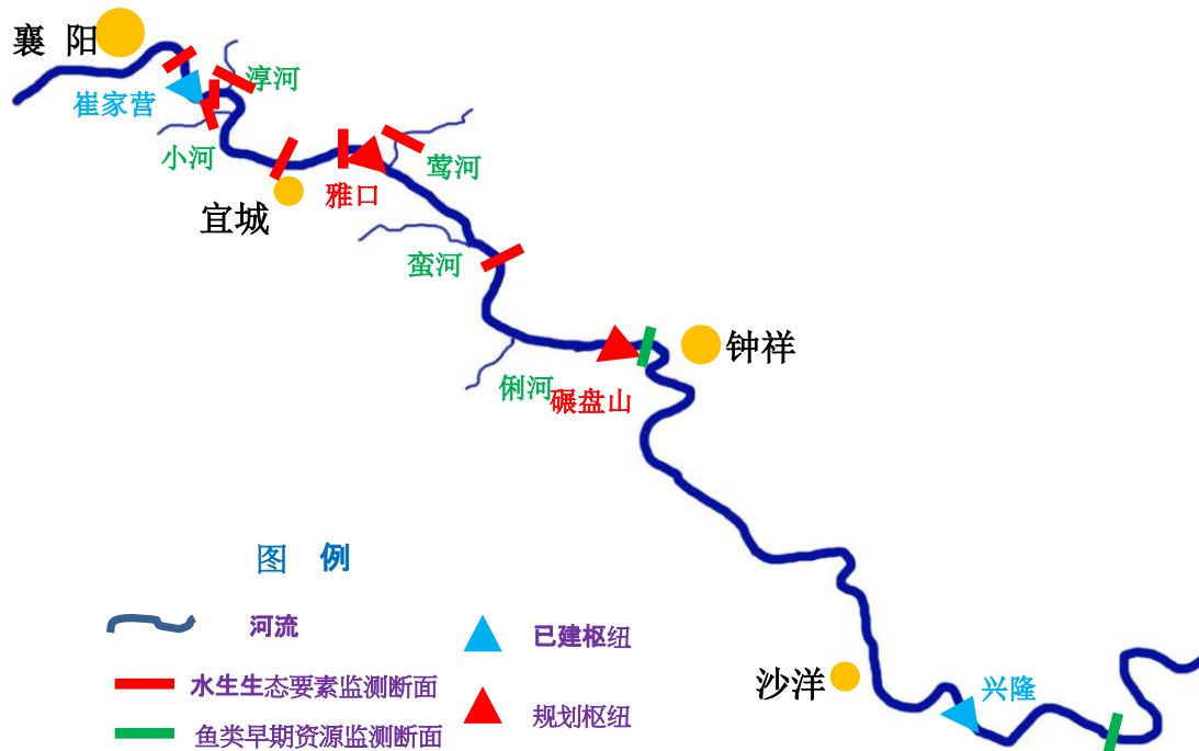
Figure 9.1.4 Monitoring sections of aquatic ecosystem
