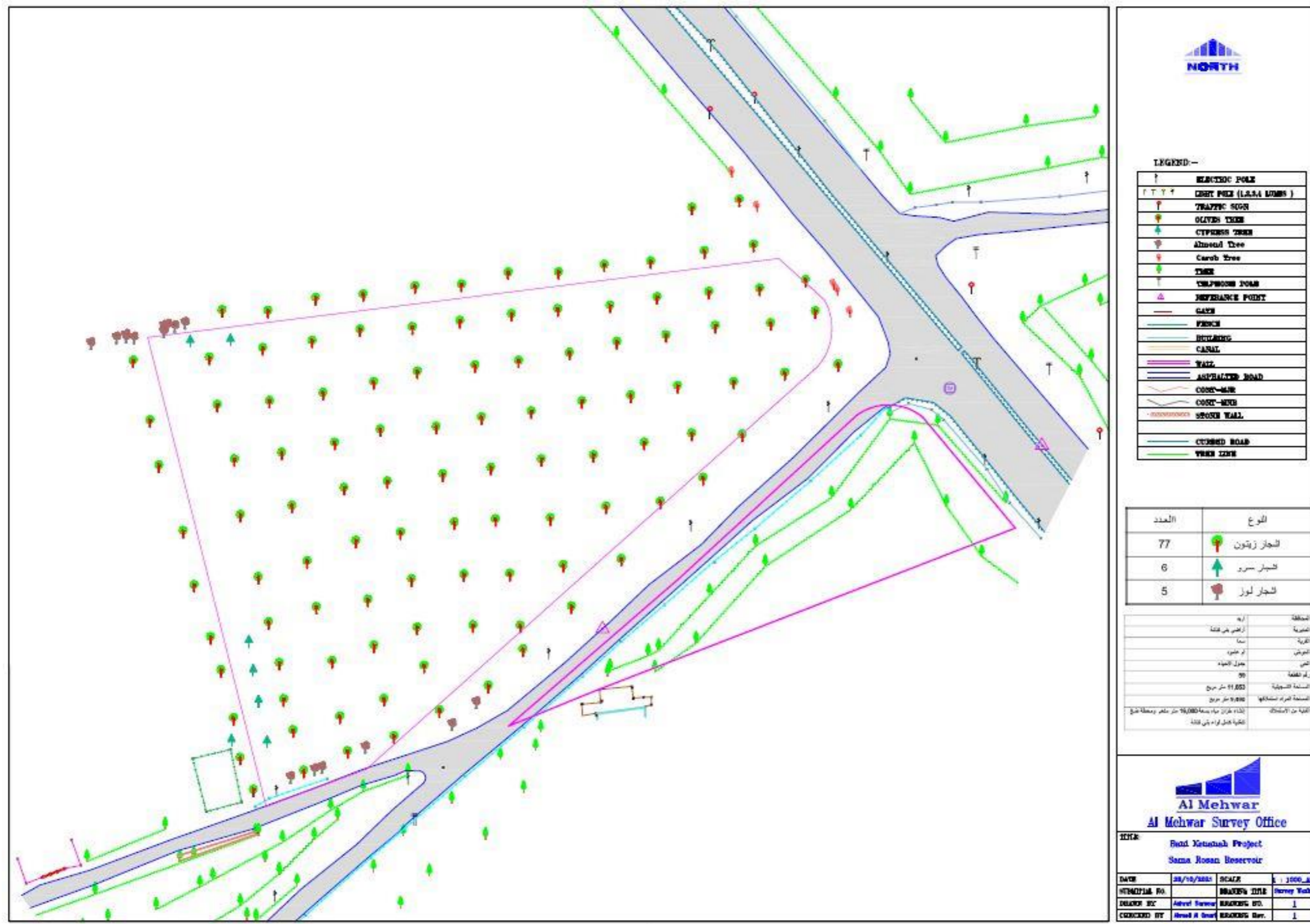
Figure 5: Trees Planned to Be Removed for the Proposed Sama Reservoir
