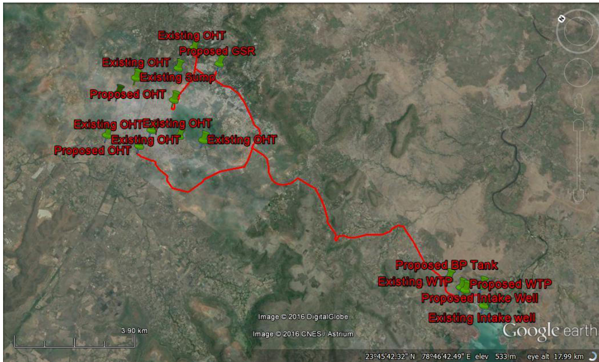
Figure 5: Locations of proposed and existing components of Sagar Water Supply on Google map
