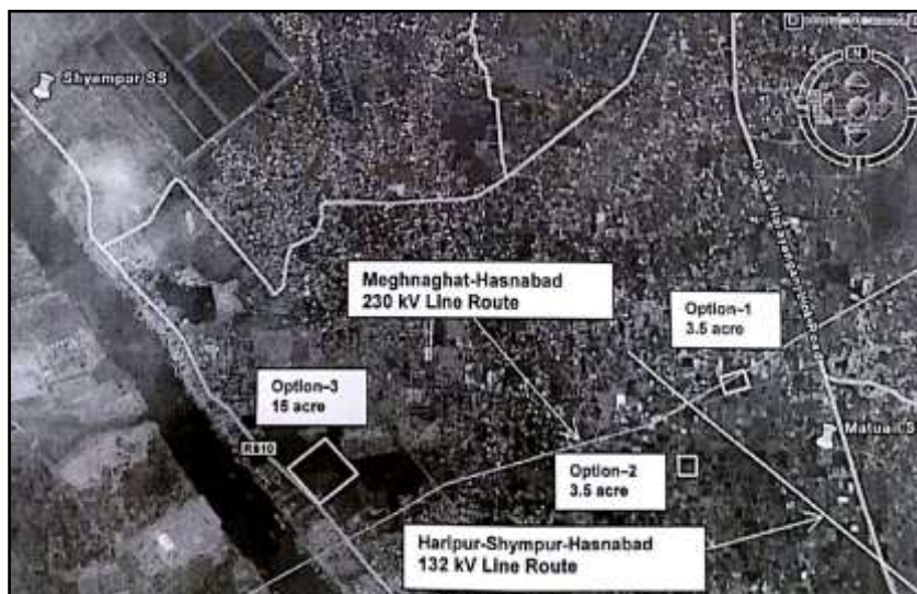
Figure 3.2 Site selection for Shyampur substation
