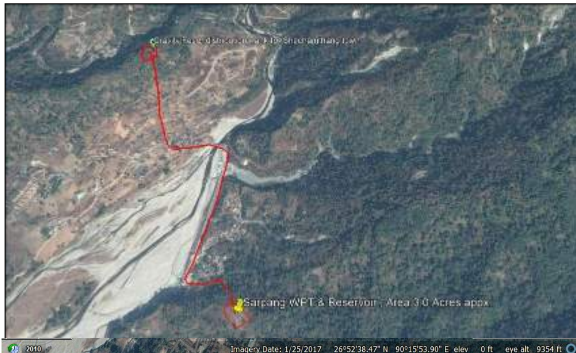
Map 7: Map Showing the Water Distribution Main Alignment from existing Water Treatment Plant to Shechamthang (2.98km)
