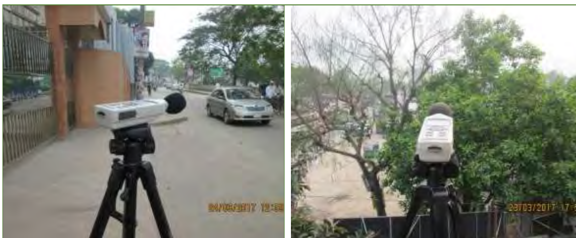
Photograph 7: Monitoring of Ambient Noise Level at Project Area
