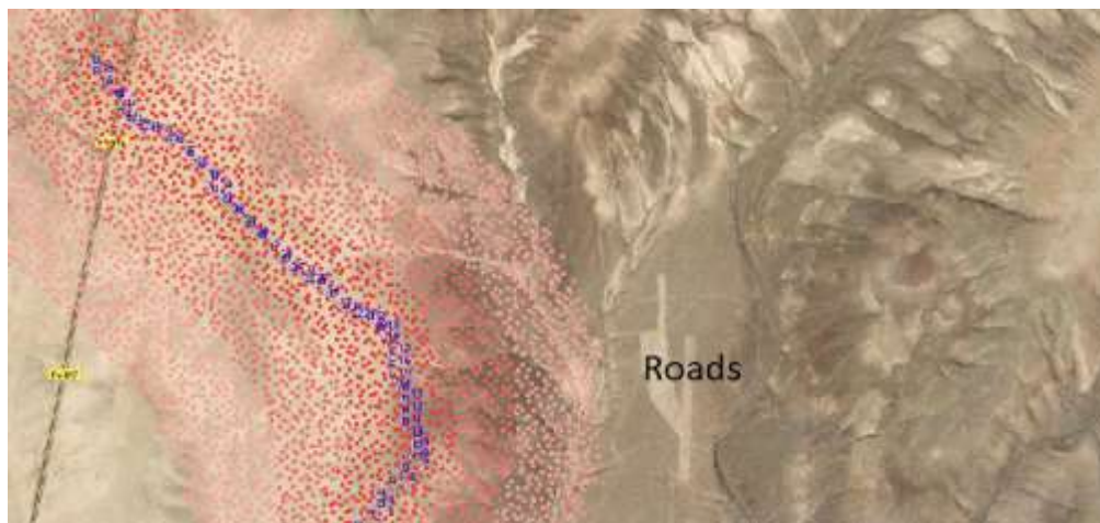
Figure 2: A typical noise intensity output in CUSTIC 3.2 for a typical road using line noise source.
