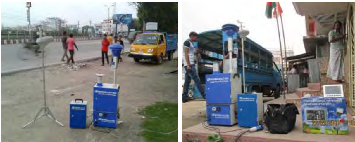
Photograph 5: Air quality measurement at the Project Road
