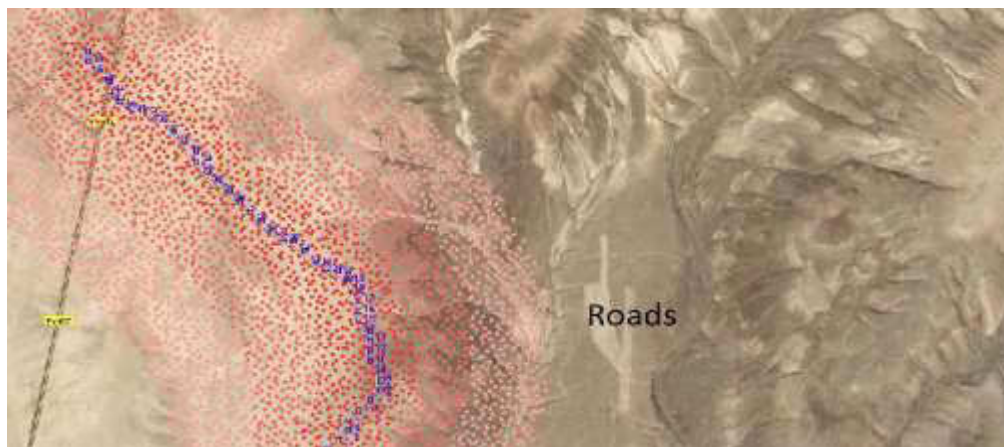
Figure 2: A typical noise intensity output in CUSTIC 3.2 for a typical road using line noise source.
