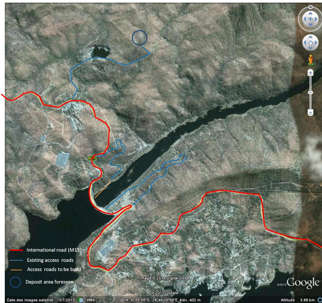
Figure 4: Access roads on site
