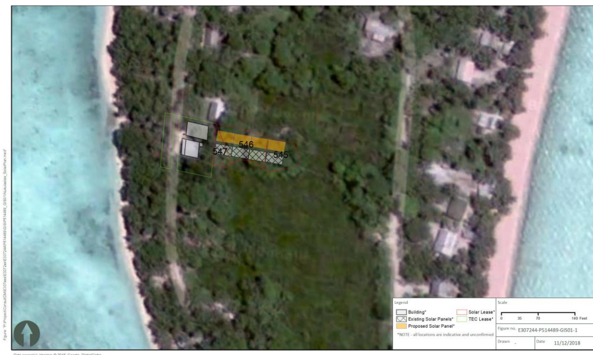
Figure 2. Nukulaelae with overlays showing locations of power station (white rectangle), existing solar array (grey hatched rectangles), proposed new station building (grey rectangle), and additional 44.8 kWp PV array (yellow rectangle). Existing lease boundaries for the powerhouse are shown in green, and existing lease boundaries for the solar PV are shown in red.
