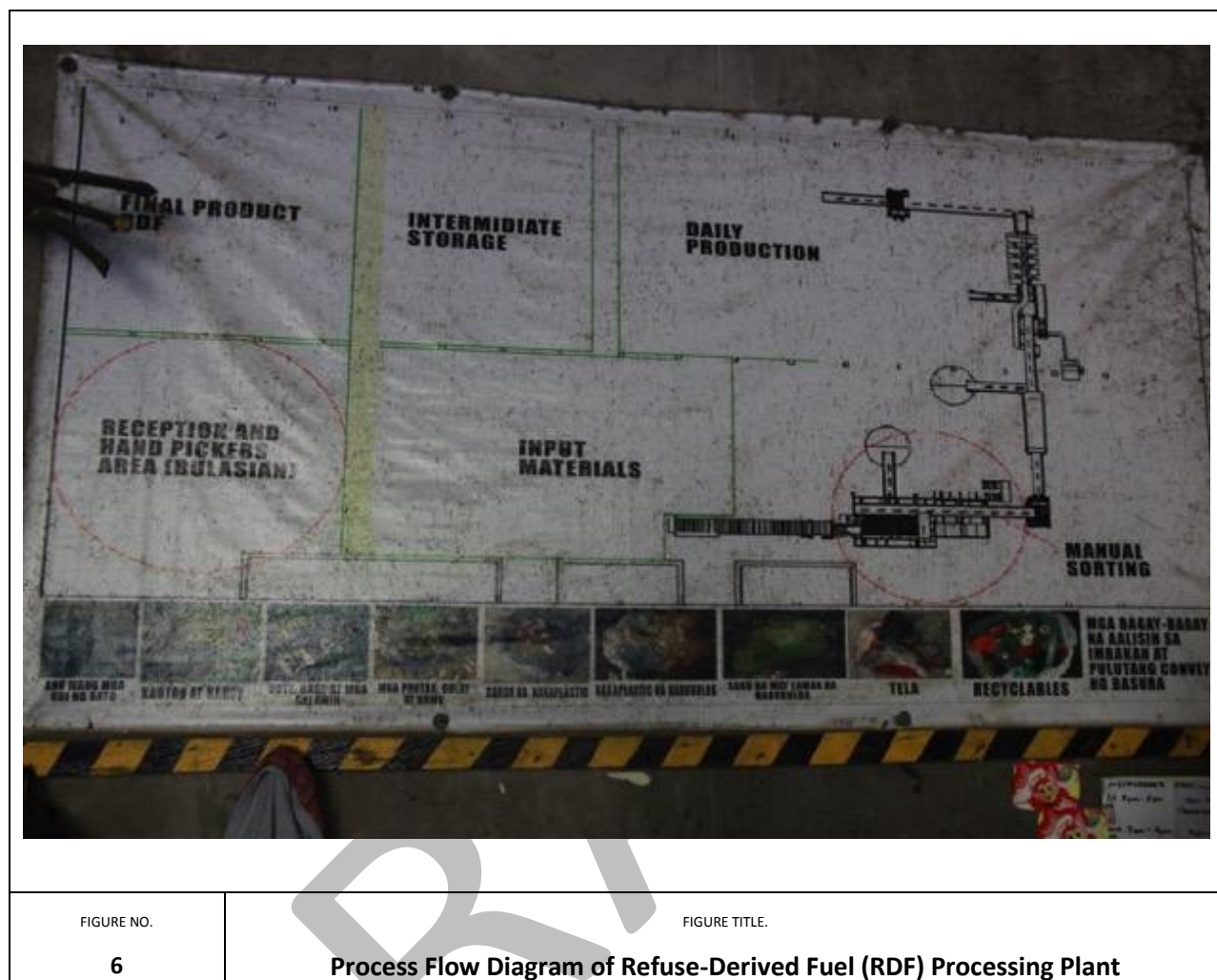
Figure 6: Process Flow Diagram of Refuse-Derived Fuel (RDF) Processing Plant
