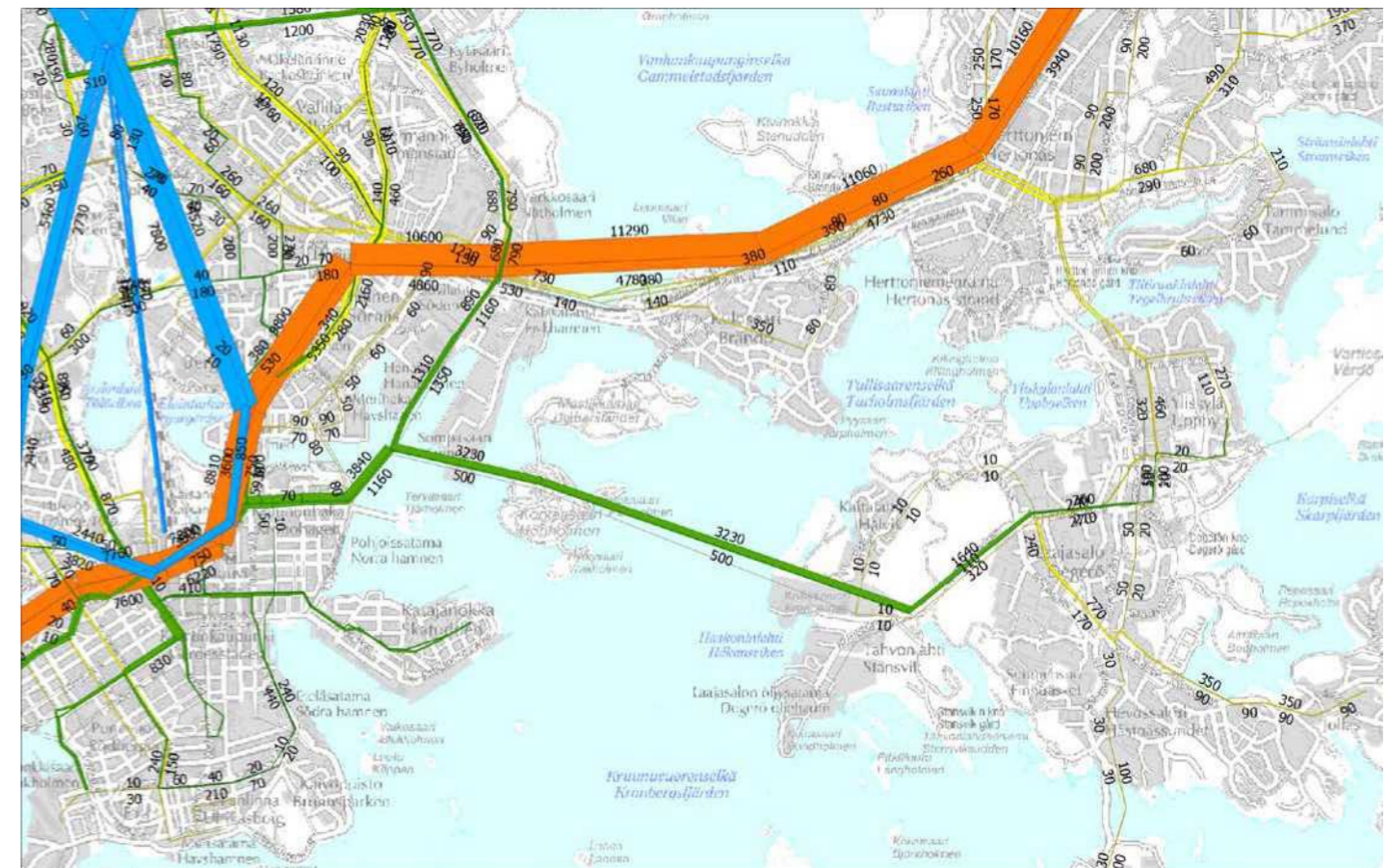
Figure 9.6. Passenger numbers in 2035 morning peak hour under the tram and vehicle bridge option.
