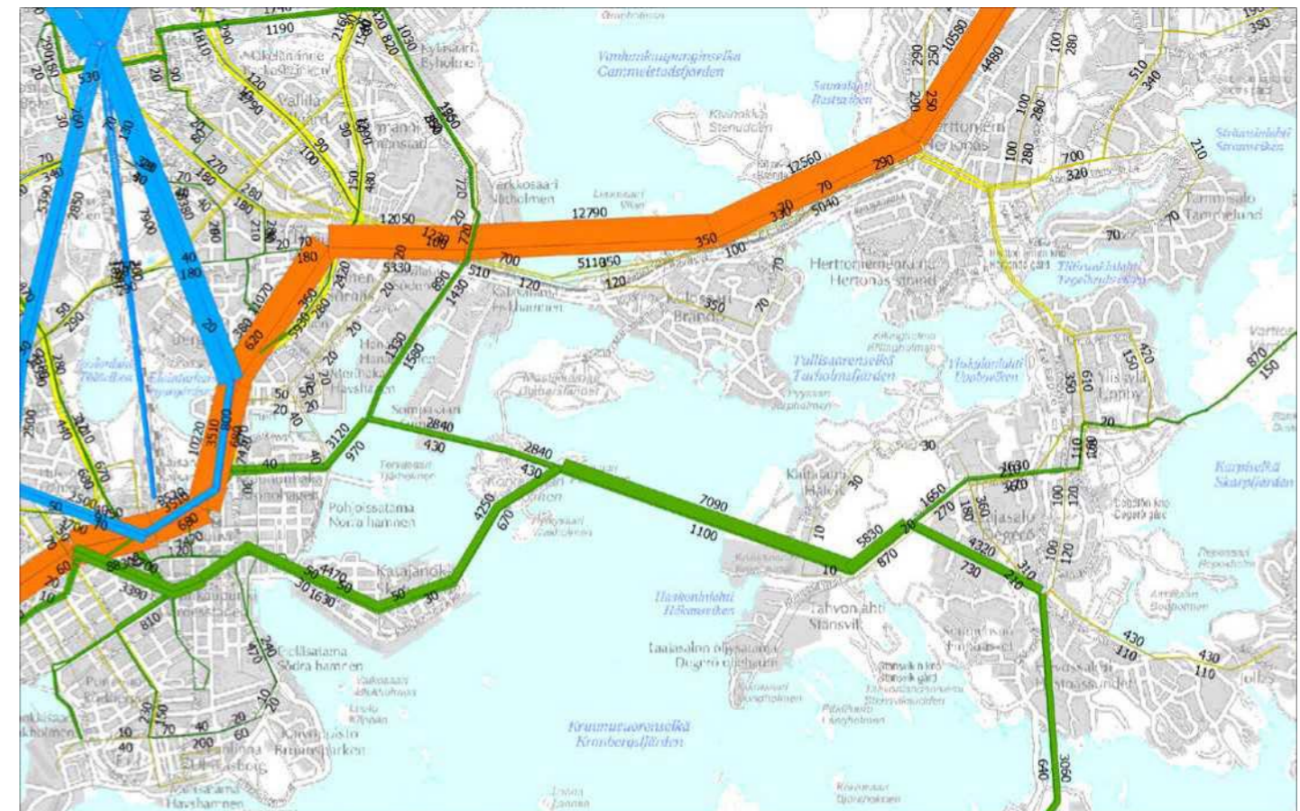
Figure 9.41. Passenger numbers in 2035 in the case of Santahamina and Vartiosaari by a quick-track
