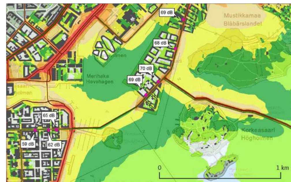
Figure 9.63. Comparison of options VE 0 (upper) and VE 8 (lower) with the areas of Kruunhaunha, fishing port and High Island. The noise levels L_{Aeq} shown in the images during the day from 7 a.m. to 22 a.m. and the maximum noise levels on the façades in the phone
