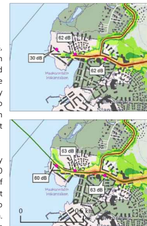
Figure 9.59. Comparison of options VE 0 (upper) and VE 1 (lower) in the area of Kruunu Mountains. The noise levels L_{Aeq} shown in the images during the day from 7 a.m. to 22 a.m. and the maximum noise
