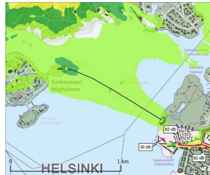
Figure 9.61. Comparison of options VE 0 (upper) and VE 3 (low) in areas adjacent to the bridge. The noise levels L_{Aeq} shown in the images during the day from 7 a.m. to 22 a.m. and the maximum noise levels on
