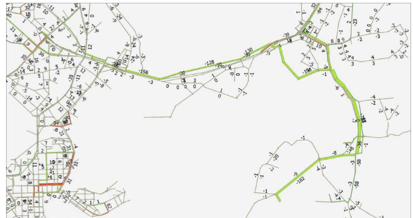
Figure 9.13. Difference in traffic volume in 2035 morning peak hour under the tram-hour option compared to option 0.
