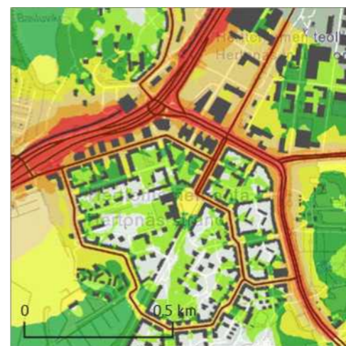
Figure 9.65. Comparison of options VE 0 (upper) and VE 8 (low) in the Herttoniemi area. The noise levels L_{Aeq} shown in the images during the day from 7 a.m. to 22 a.m. and the maximum noise levels on the façades in
