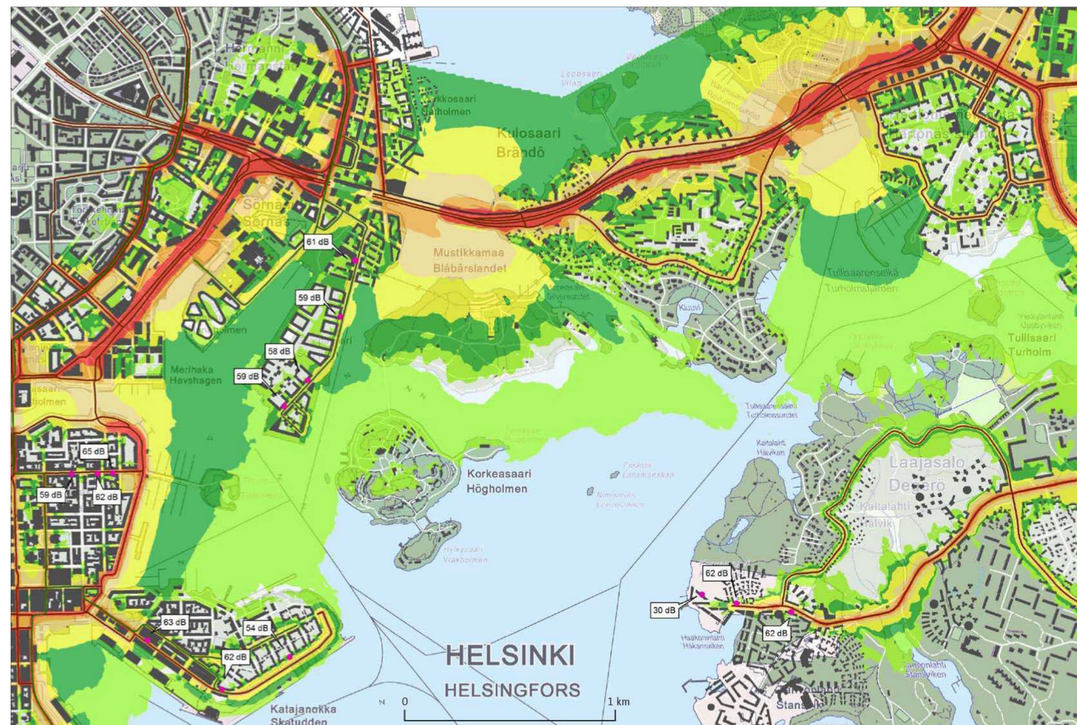
Figure 9.57. Noise levels L_{Aeq} by day from 7 a.m. to 22 a.m. in option 0. The highest noise levels calculated on the façades in the area are
