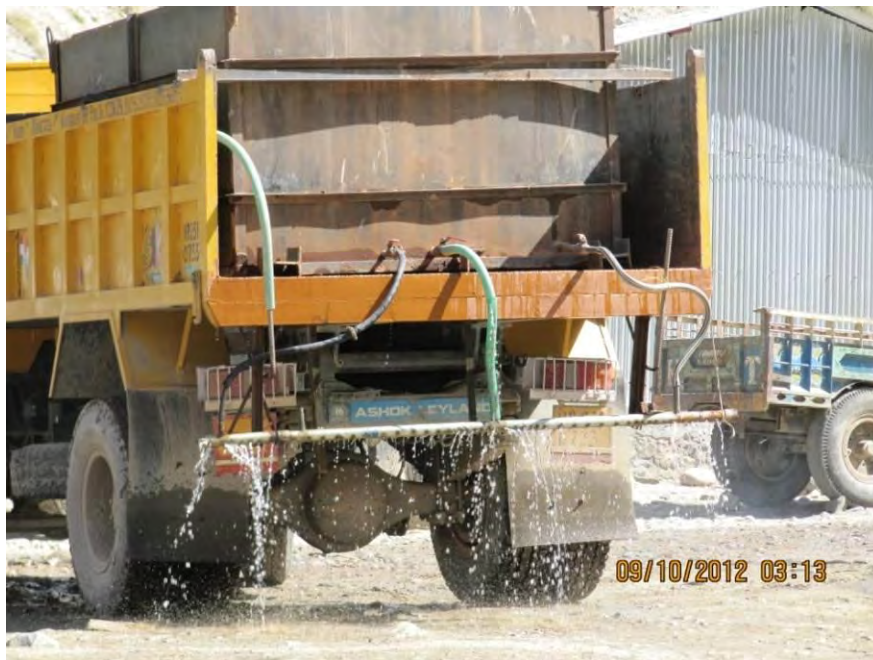
Figure 5-3: Water sprinkling system mounted on a truck
