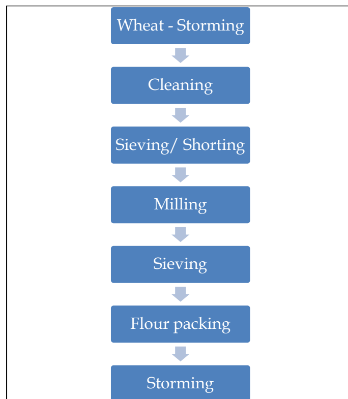
Exhibit 9. Process Flow Diagram of Flour Mill
