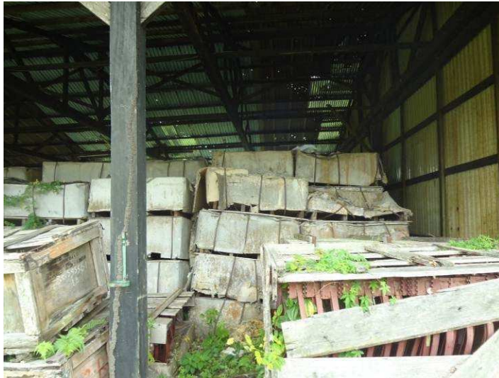
Photograph 5: Expired drilling mud material stored on unpaved ground
