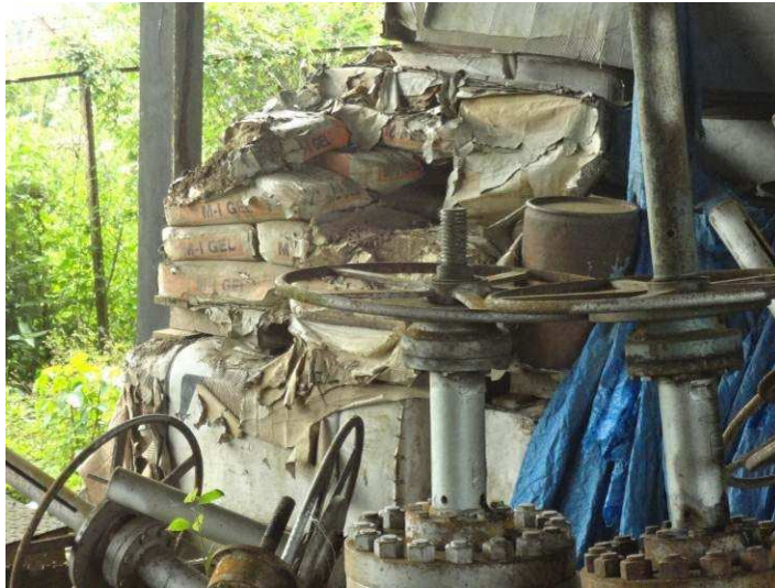
Photograph 6: Expired drilling mud material stored on unpaved ground
